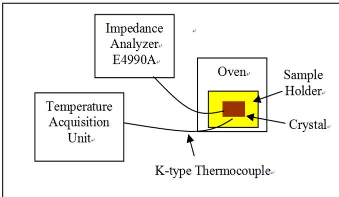
Fig. 1: Set up for phase transition measurement
