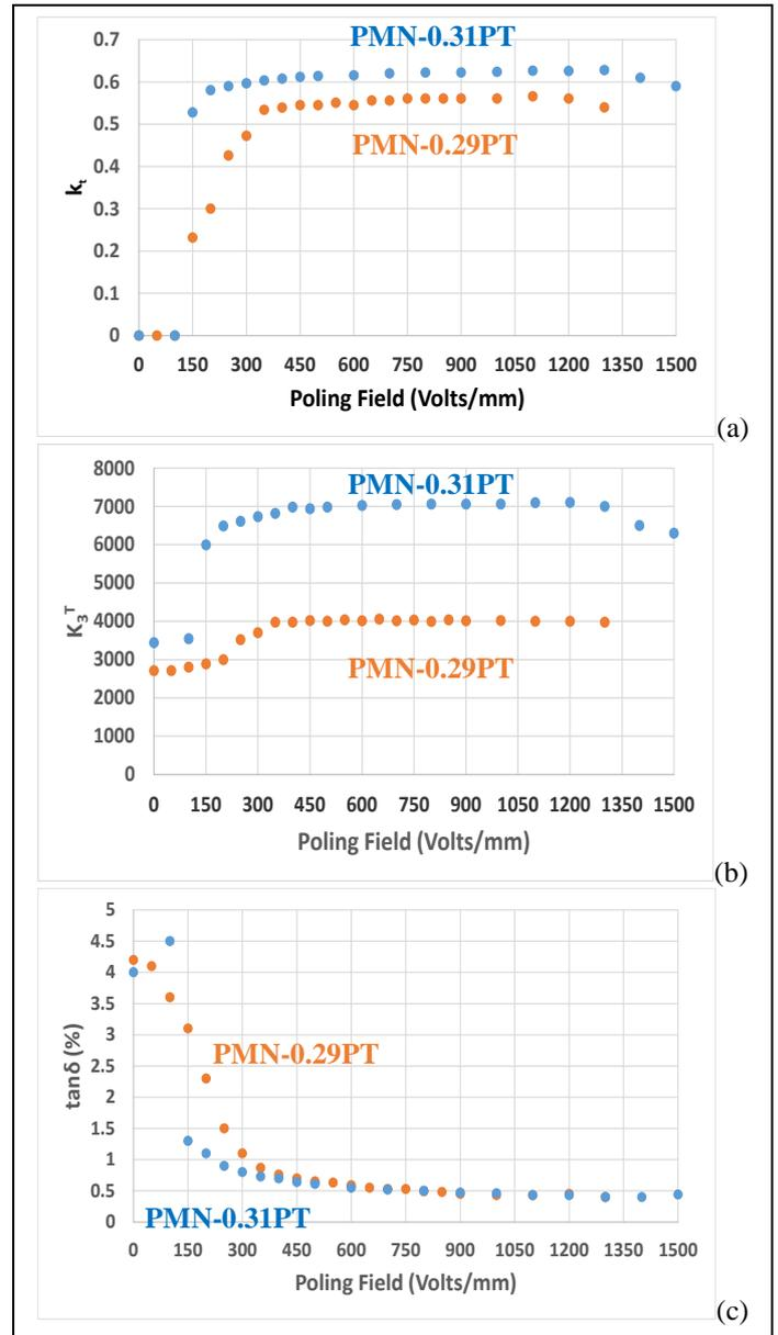
Figure 2: Poling Effects on (a) Plate-mode Electromechanical Coupling Coefficient  $k_t$ , (b) Dielectric Constant  $K_3^T$ , and (c) Dielectric Loss  $\tan \delta$  of PMN-0.29PT and PMN-0.31PT Crystals
