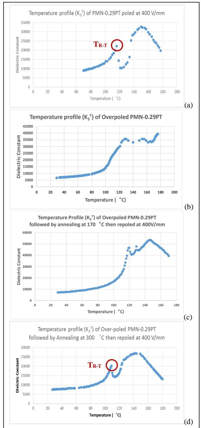
Figure 3: Dielectric Constant vs. Temperature profile of a PMN-0.29PT plate sample (a) poled at 400 V/mm; (b) over-poled at 1500 V/mm; (c) over-poled at 1500 V/mm, annealed at 170 °C for 1 hr, then re-poled at 400 V/mm; (d) over-poled at 1500 V/mm, annealed at 300 °C for 1 hr, then re-poled at 400 V/mm.
